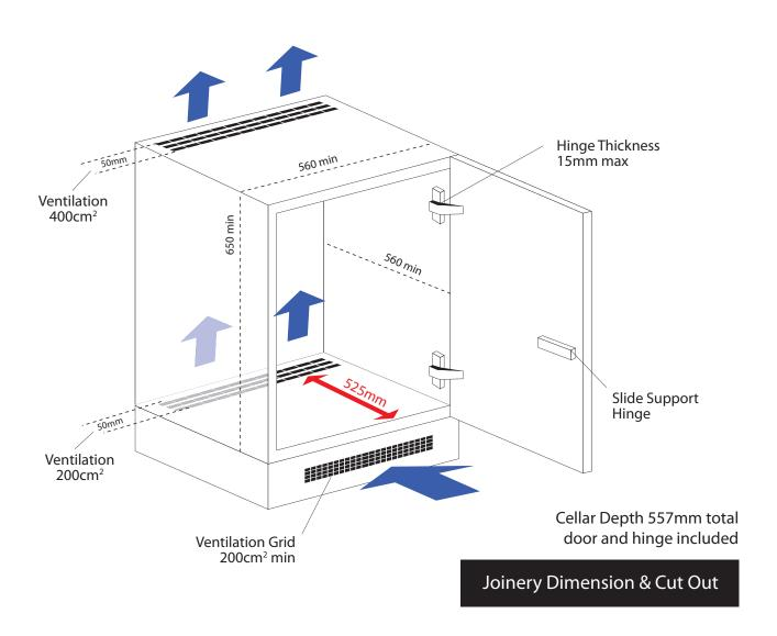
Note: Dimension of Studio: H640xW540xD557mm. Actual appliance measurements, specifications and ratings may vary slightly due to technical improvements and slight manufacturing differences. When dimensions are critical it is important that an effective check be made and the accompanying instructions and installation manual be read.
